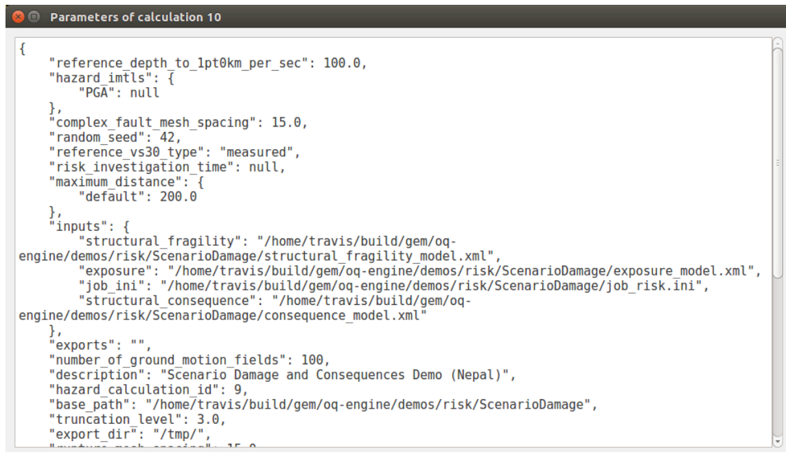
Fig. 12.4: Example showing parameters of a OQ-Engine calculation
